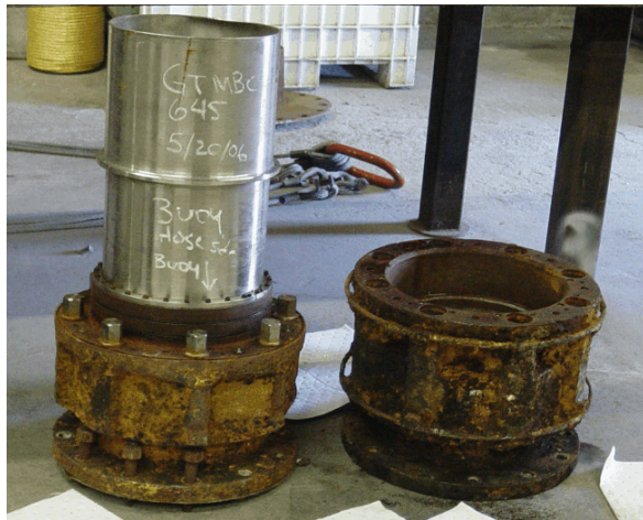
Figure 6a and 6b. The subject GTC in Hawaii. Both halves are shown in 6a. The shutoff valve in the ship end of the GTC can be seen in 6b.
