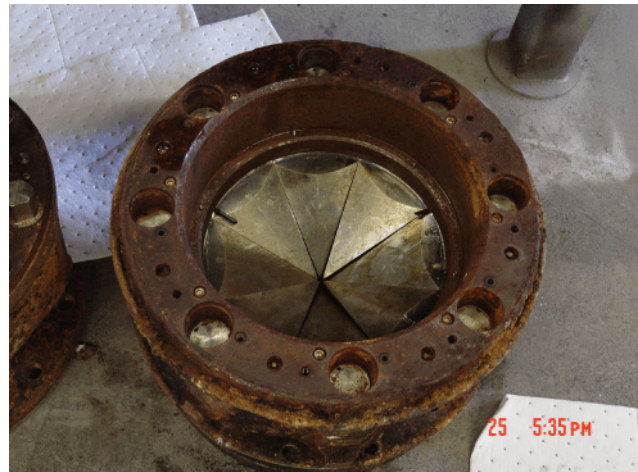
Figure 6a and 6b. The subject GTC in Hawaii. Both halves are shown in 6a. The shutoff valve in the ship end of the GTC can be seen in 6b.
