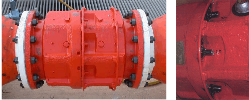
Figures 2a and 2b. Gall Thomson breakaway in a hose string on left and closeup of installed breakaway studs on the right.
