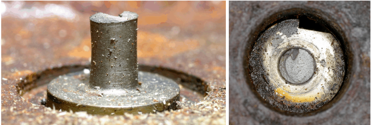
Figure 14a and 14b. Breakstud #3 fractured through the radius at the end of the reduced section.
